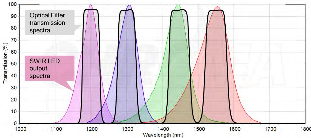
These filters remove the overlap present with the SWIR LEDs, increasing image contrast by removing more unwanted light from each image.
