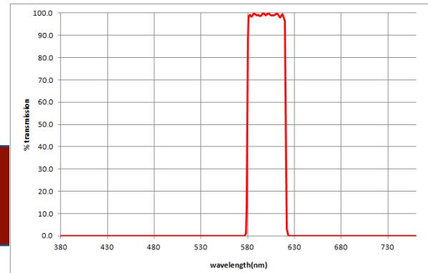
A spectral plot shows % transmission as a function of wavelength and represents the percentage of **energy** that gets through the filter -- what is not allowed to transmit is either **absorbed** or **reflected**.  $T + A + R = 100\%$
